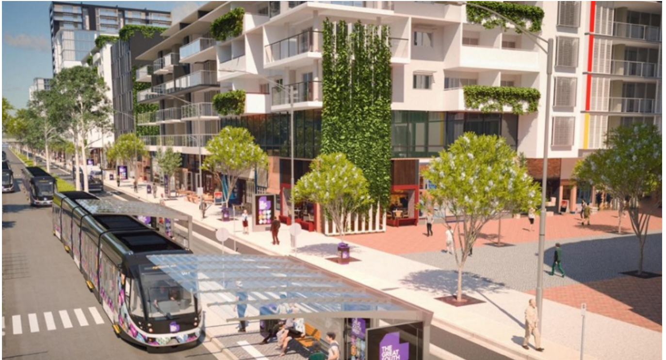
Figure 3.12: Mid-tier Transit corridor in concept using a trackless tram and integrated station precincts as illustrated by City of Liverpool in Sydney for SBEnrc project.
