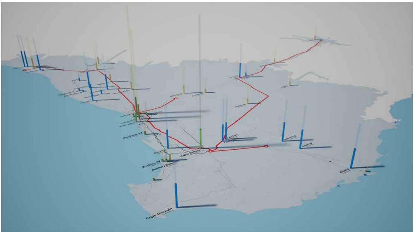
Figure 5.13: SWIS Nodal Map: Potential network augmentation to 2042
